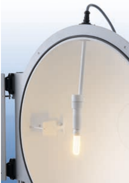
ISP1000 opened with lamp post suspended
